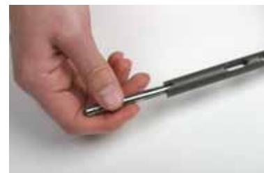
Insert is correct. It can be screwed in and only wobbles slightly
